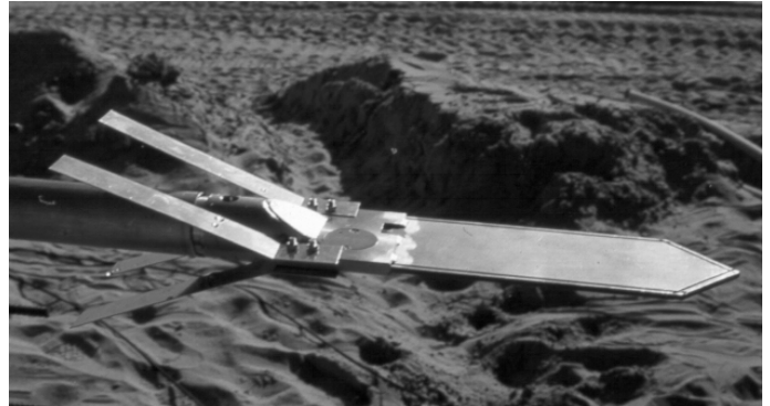
Figure 6. Earth pressure cell with modified wings
